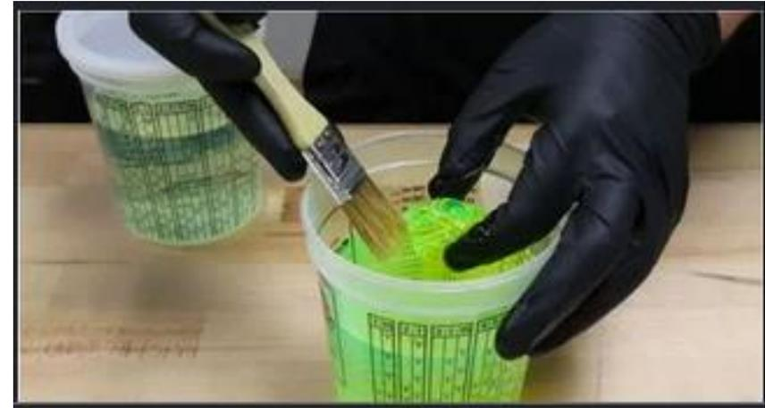
**Rinsing and cleaning for 3d Printed parts in Isopropyl Alcohol**
