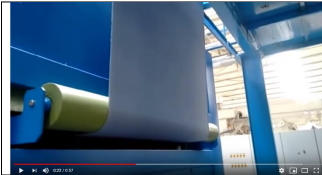
Dhall Thermosol Dyeing Pad Dry Range at Saygindima Textile
