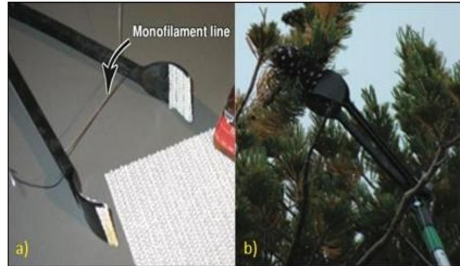
Figure 3: a) Tree tong with cord for opening and closing;
