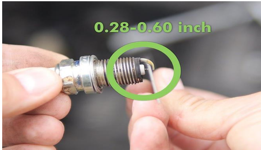
4 Measure the gap of the spark plug.
