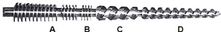
Figure 11.52. Cross section of conical twin screw extruder showing zones for (A) feed and plastication, (B) restrictive, (C) devolatilization and (D) metering.
