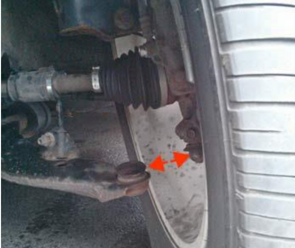
This ball joint has separated while driving
