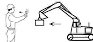
Move Load Out Horizontally With either arm extended, hand raised and open toward direction of movement, move hand in direction of required movement.
