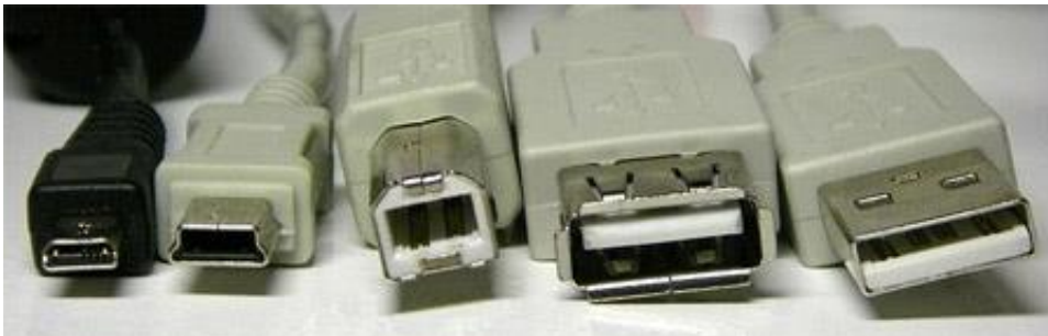
From left to right: micro USB, mini USB, type B standard USB, and type A standard USB (both female and male)
